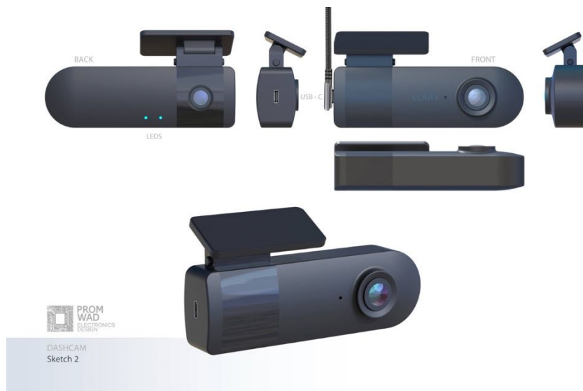
A dashboard camera prototype based on Telit Cinterion modules
