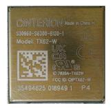
Operating frequency bands and related max radio-frequency power transmitted: LTE CAT NB1/2: (B1, B3, B8, B20) 20dbm +2/-2dB; (B28) 20dbm +2/-2.5dB LTE CAT M1: (B1, B3, B8, B20) 20dbm +2/-2dB; (B28) 20dbm +2/-2.5dB
